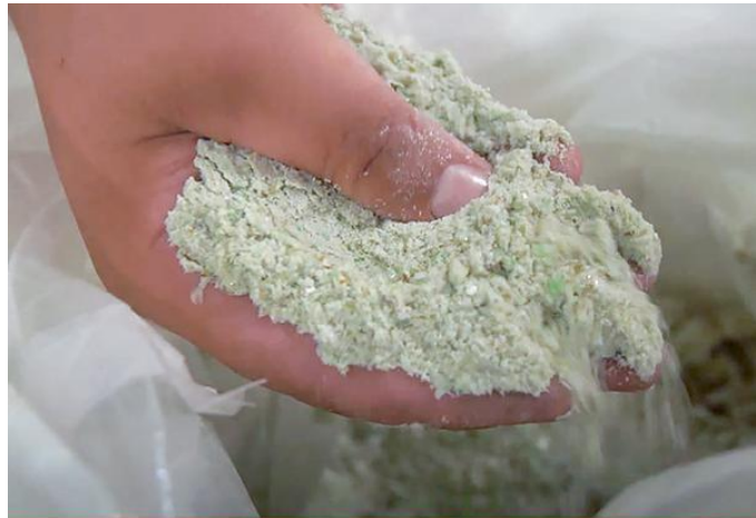
Figure 6. Glass Crushed to Sand (Courtesy Aqua Tools)
