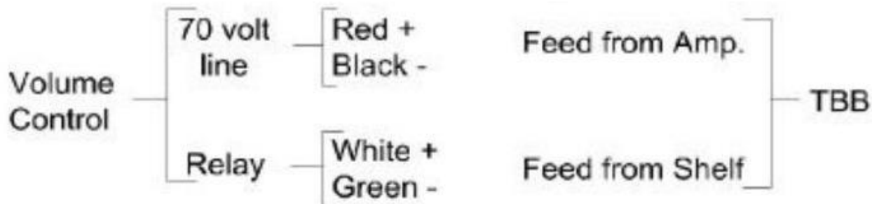
Figure 2: Supplemental schematic detail illustrating 70-volt line connections and relay interface. The diagram identifies a 70-volt line with Red (+) and Black (–) conductors as the feed from the amplifier to the TBB, and a relay connection with White (+) and Green (–) conductors as the feed from the equipment shelf. Volume control and feed paths are labeled to clarify signal routing to the terminal block.
